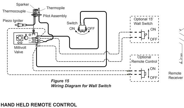
The remote control receiver may be installed in the control panel by removing the ON/OFF switch and the knock-out plate. Slide the receiver into the space where the knock-out plate was removed. Refer to remote instructions for wiring and operation.
